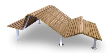
Each module is composed of a tubular steel frame, section 50x30 mm and of flat iron, section 50x8 mm entirely hot-dip galvanized and assembled with Nordic pine wood planks pressure treated, section 60x30 mm. The modules are assembled together by forming a deckchair on one side with leg support and a classic seat on the other side. Supplied in an assembly kit with galvanized steel bolts. Anchorage system: to be fixed on the ground.
