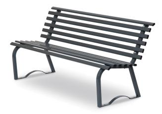
The structure consists of 2 tubular steel supports with a square section 30 x 30 mm with an anatomical shape, 150 cm in length. It consists of twelve steel bars with an oval section 40x20 mm equipped with plastic caps at both ends. Fastening system to the supports through galvanized steel bolts. Anchorage system: to be fixed on the ground. Supplied in an assembly-kit. Entirely galvanized, powder coating at 180°C.
